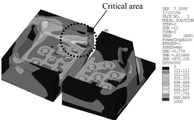
Fig.6. Critical area on coil block shoulder (von Mises stresses in coil blocks at 120% of operational design load at 4K shown)
